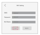
3.7 The system starts to search the device, it takes about a few seconds, when the pop up a message says "Linked module" and the LED of WIFI module stops blinking and finally stay on green, the configuration is finished and successful. Click "OK".
