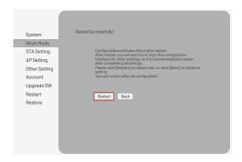
4.7 If the green light of the WIFI module is always on, it indicates that the connection with the router is successful. Close the browser and, the configuration is completed.
