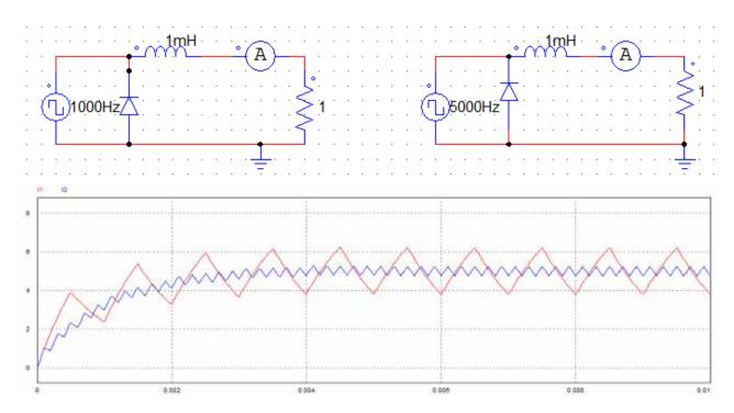
Equally increasing the invert frequency and reducing the inductance value can obtain the same amplitude ripple current, and the high frequency can be stabilized faster.
