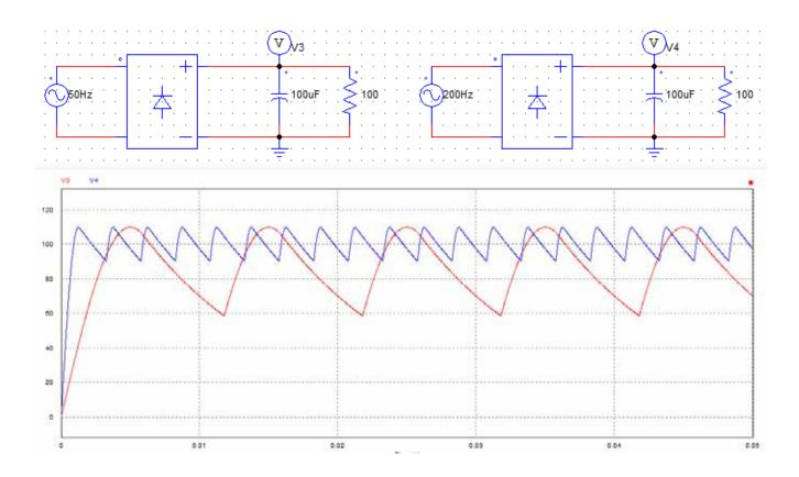
Increase the invert frequency in the same proportion and reduce the capacitance of the capacitor to obtain the ripple voltage of the same amplitude.
