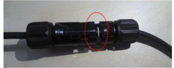
The terminals are not connected tightly
