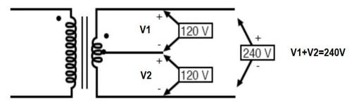
As the nominal output voltage of most Renac Power single-phase solar inverters is 230V with neutral wire, Inverter will not work if connected as usual.
