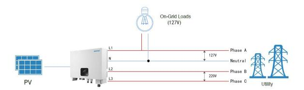
To fit such electricity system, Renac Power provides a solution by LV version Grid-tied 3phase solar inverters NAC10-20K-LV series, which include NAC10K-LV, NAC12K-LV, NAC15K-LV, NAC15K-LV, which could use with both Star Grid or Delta Grid by commissioning on inverter display (just need to set inverter safety as "Brazil-LV").
