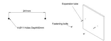
Step 2: Place the inverter on the wall-mounted bracket and install the fix screw.
