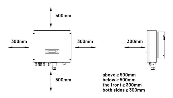
• When installing several inverters, reserve enough clearance around the inverters to ensure sufficient space for heat dissipation.
